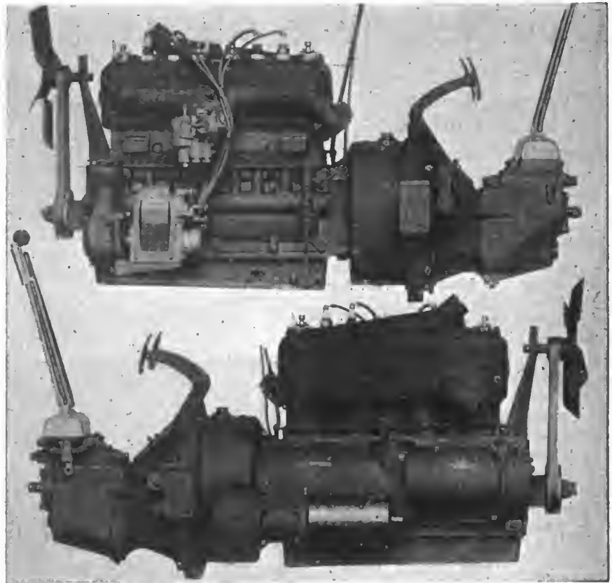
Both sides of the four-cylinder L-head unit power plant used in the 1917 Princess. The engine has a bore of 3\frac{3}{4} and a stroke of 4\frac{1}{4} in., giving a piston displacement of 187.9 cu. in. and a formula rating of 22.5 hp.
